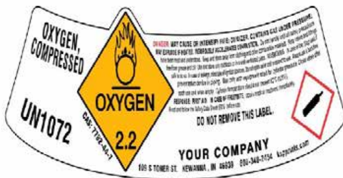
Figure 5: Example of an Oxygen cylinder shoulder label for transport and use
